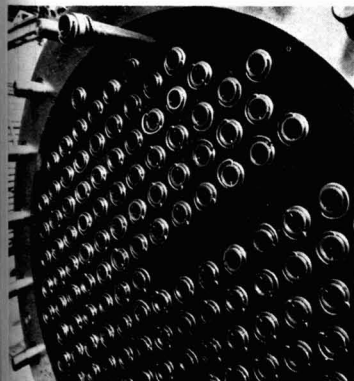
Coaxial juice heater (upper tube sheet)
