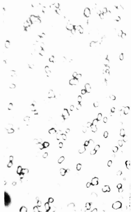
Fig. 4. Photomicrograph of 2nd carbonatation precipitate from frost-damaged beet stored for 7 days after thawing ( \times 1000 )
