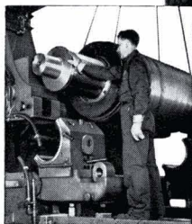
Patented side-cap construction permits fast vertical roll removal.
