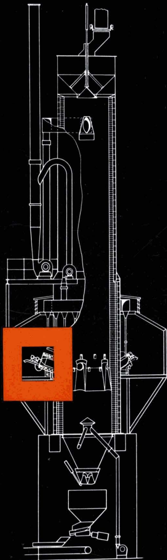
The oil carburetting unit, key to the West's lime kiln's well-proven Catagas oil firing system.
