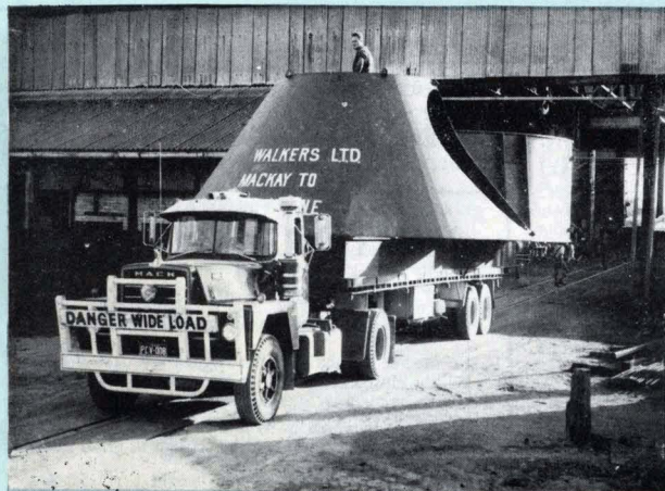
TOP CONE OF A 24,000 SQ.FT. EVAPORATOR LEAVING MACKAY FOR PROSERPINE MILL, 90 MILES FURTHER NORTH.
