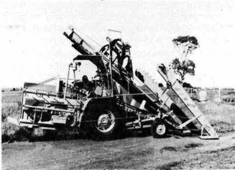
Fig. 3. Toft J250 whole-stalk harvester
