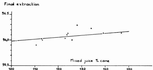
Fig. 4. Effect of draft on final extraction
