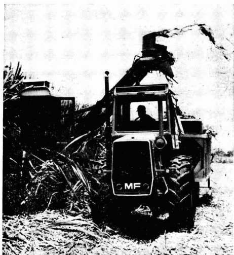
2. 'Big Little Red'. The MF 102, built to handle up to 15,000 tons of cane in a season. Picture shows the MF 102 cutting green cane for seed at Cambalache, Puerto Rico, 1973. On this occasion it is accompanied by the 4 wd MF 1200 tractor pulling a 3-ton chopped cane planter.
