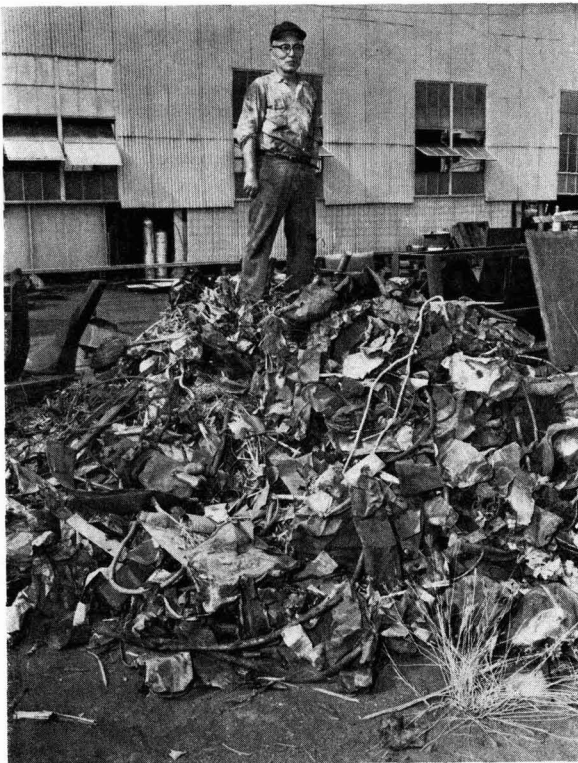
Fig. 1. Workman standing on top of mountain of crusher-damaging tramp iron extracted from sugar cane by magnetic separators supplied by Eriez Magnetics
