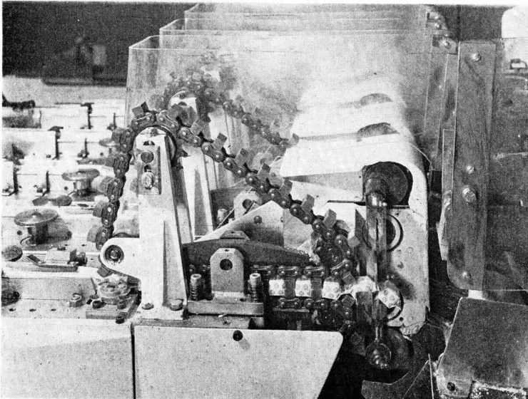
Fig. 3. The portion-wrapper wraps 3000 double-cube portions per minute. The wrapping paper is formed into a tube, which is cold sealed and cut between each pair of sugar cubes.
