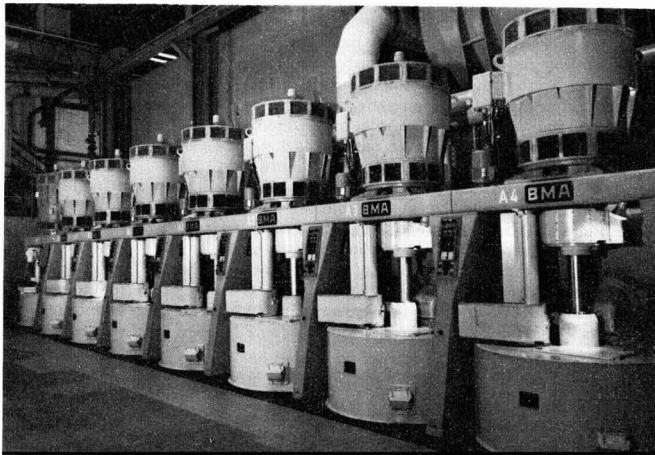
BMA centrifugals: (left) a belt-driven machine of 1900, (right) a modern fully-automatic "Variant"-type battery
