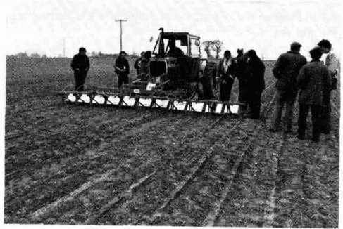
Fig. 4. Inter-row 11-row crop sprayer, W.F. Engineering
