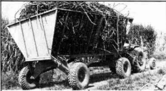
This 4-wheeled trailer transfers appr. 1.5 ton to the pulling Massey-Ferguson Tractors rear- axle. - (Bunger-Trailer-System).
