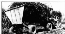
This 4-wheeled trailer transfers approx. 1,5 ton to the pulling Massey-Ferguson Tractors rear-axle. - (Bunger-Trailer-System).
