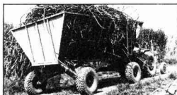
This 4-wheeled trailer transfers approx. 1.5 ton to the pulling Massey-Ferguson Tractors rear-axle - (Bunger-Trailer-System).
