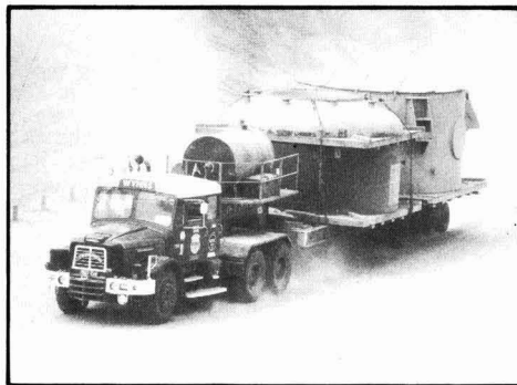
"Out-of-gauge" equipment being brought 1200 km across the desert from Port Sudan to site on heavy-duty articulated trailers. 1500 tonnes of such equipment was brought to site in this way.
