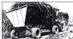
This 4-wheeled trailer transfers appr. 1.5 ton to the pulling Massey-Ferguson Tractors rear-axle. - (Bunger-Trailer-System).
