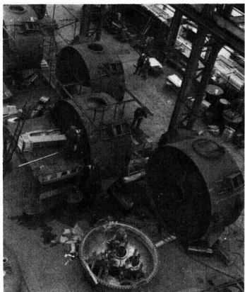
Tube expanding Kenana evaporator bundle
