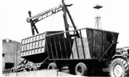
Bü-88 Super Tandem Combination for discharge of 15 ton cane. (Gantry or crane-beam.)
