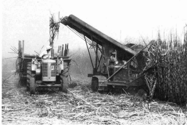
Fig. 1. The first whole-stalk cane harvester made in Brazil
