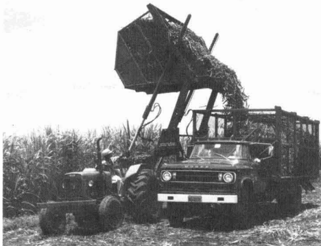
Fig. 6. Unloading a VT-5 infield unit into a road truck
