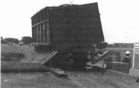
Fig. 7. The Santal TSM side-unloading system
