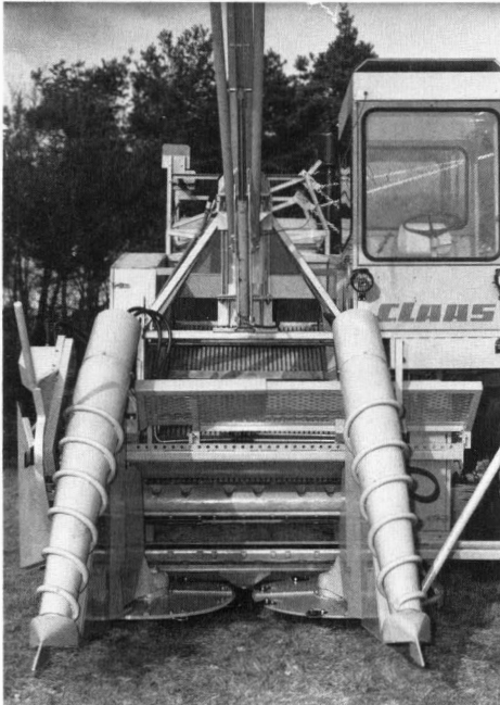
Fig. 1. The intake system of the Claas CC 140Q green cane harvester is provided with rotating scrolls and shoes which can be moved to vary the throat between 1400 and 1950 mm, two rotating disc base cutters, a vertically rotating double knife (left) to cut off overhanging stalks, and the toppler
