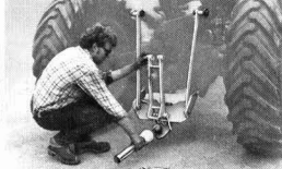
Bü-Ball-Coupling complete for hitching by tractors standard hydraulic arms.
