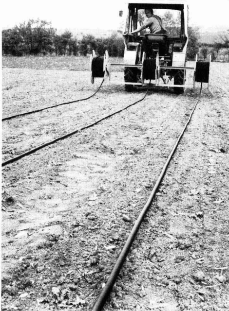
Fig. 3. The fully-mechanized tractor-mounted coiling unit has proved to be especially useful for agricultural areas with large drip irrigation installations
