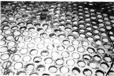
Fig. 4. Scaling of fourth body prior to cleaning and before Miltreat trials
