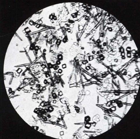
Scale formation in untreated water.
