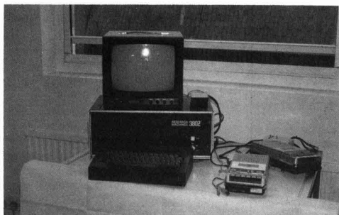
Fig. 3. Microprocessor-based computer and V.D.U. used in the Newark laboratory data recording and calculation system
