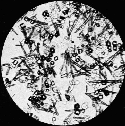
Scale formation in untreated water.
