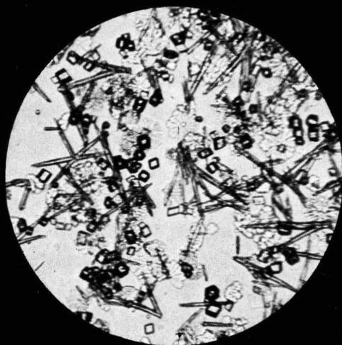
Scale formation in untreated water.
