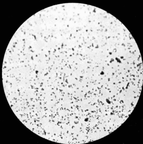
Scale formation in water treated with Miltreat S607.
