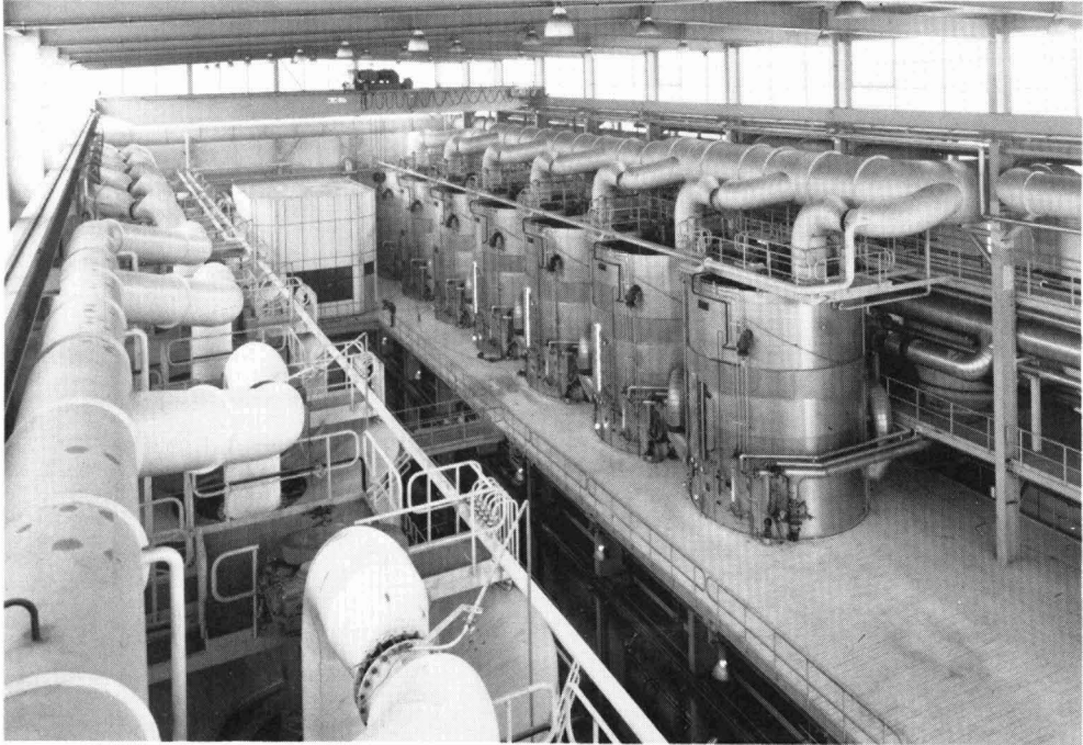
Fig. 1. The pan floor at Groningen showing the seventeen 95-tonne pans and control room
