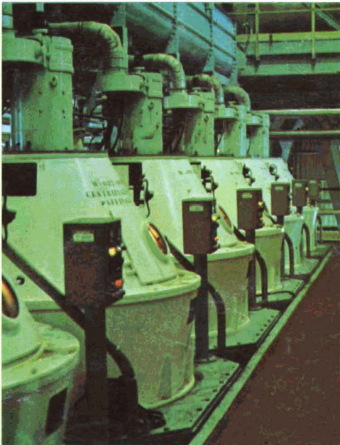
View of a battery of five Bosco B7 fully automatic batch centrifugals, D.C. driving system, for white sugar. KSAR EL KEBIR SUGAR FACTORY (MOROCCO) PROCESSING CAPACITY: 4000 TBD
