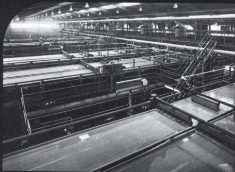
Uranium ore treatment plant including 9 vacuum belt filters, with a total working area of 846 sq.m.
