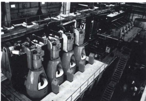
Centrifugal station of the N'Koleng, Cameroons, cane sugar factory. In the foreground, four "COMPACT 411" centrifugals. In the background, five continuous "FC 1000" centrifugals.
