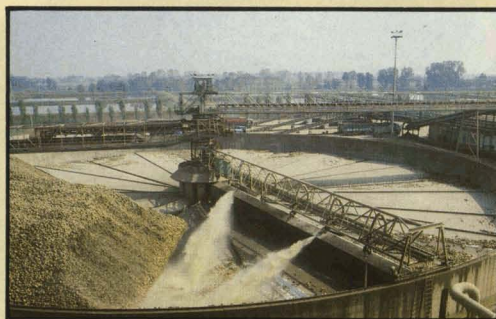
FS/Elfa Beet Silo and fluming equipment at a sugar factory in Italy.
