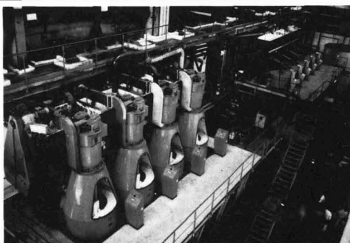
Centrifugal station of the N'Koteng, Camerons, cane sugar factory. In the foreground, four "COMPACT 411" centrifugals. In the background, five continuous "FC 1000" centrifugals.
