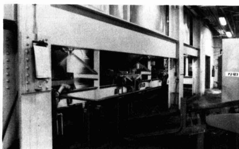
Fig. 15. Transfer of spent adsorbent from the new dewatering vessels (To be continued)
