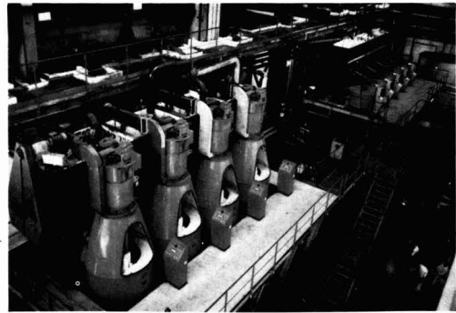
Centrifugal station of the N'Koteng, Camerouns, cane sugar factory. In the foreground, four "COMPACT 411" centrifugals. In the background, five continuous "FC 1000" centrifugals.
