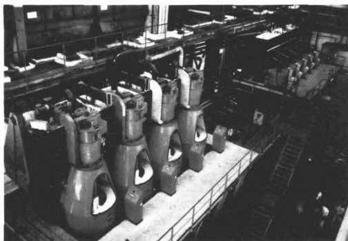
Centrifugal station of the N'Koteng, Cameroons, cane sugar factory. In the foreground, four "COMPACT 411" centrifugals. In the background, five continuous "FC 1000" centrifugals.
