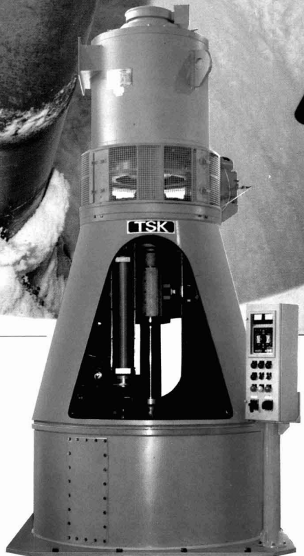
Fully automatic batch centrifugal of self-supported structure driven by brushless thyristor motor (BL Motor) in Thailand
