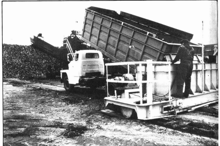
Fig. 2. For unloading semi-trailers, Michigan Sugar personnel designed this special swing-away conveyor to feed the main belt. The Link-Belt Motogear speed reducer can be seen at left of unit. This is similar to a screen drive unit, but a silicone fluid drive is not required because of low potential for jamming
