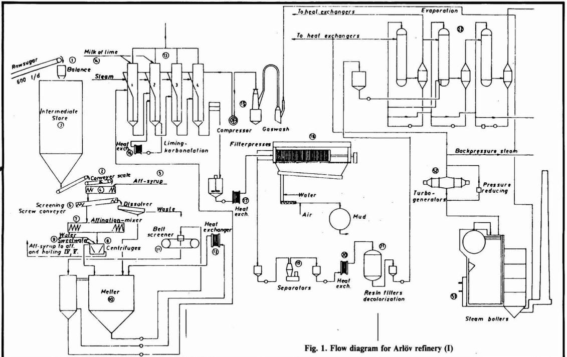
Fig. 1. Flow diagram for Arlövs refinery (I)
