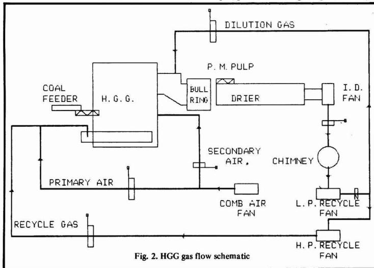
Fig. 2. HGG gas flow schematic
