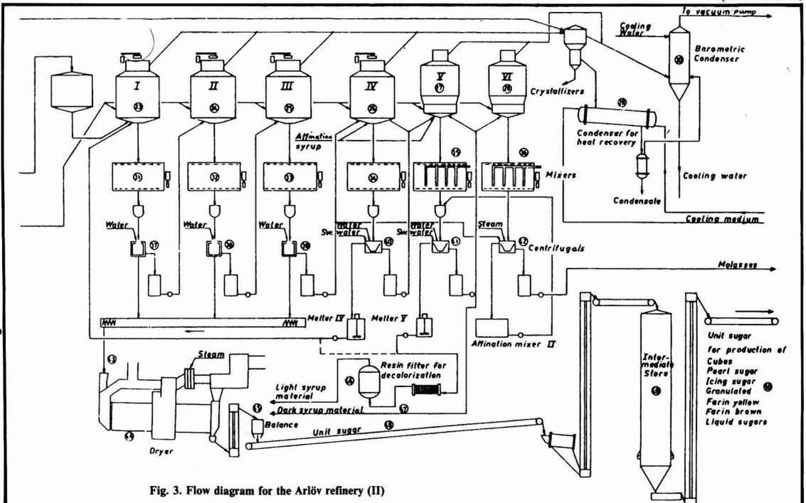
Fig. 3. Flow diagram for the Arlöf refinery (II)
