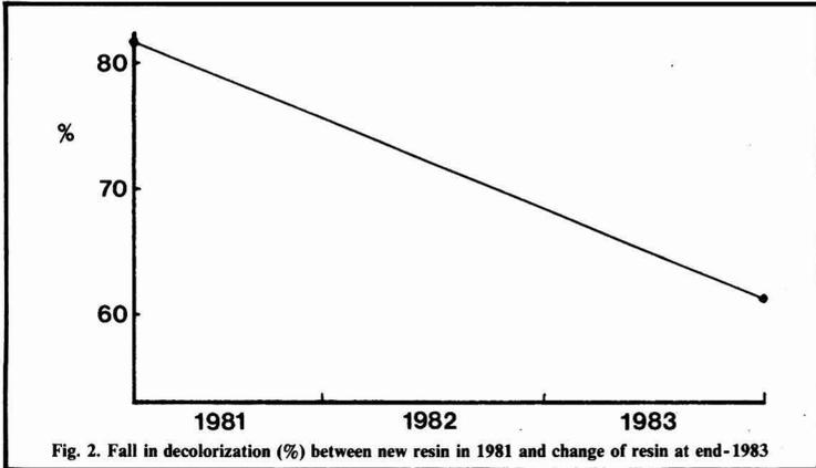
Fig. 2. Fall in decolorization (%) between new resin in 1981 and change of resin at end-1983
