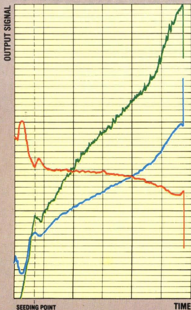
Chart showing control and reference signals over a typical batch boiling cycle – white sugar beet massecuite.
