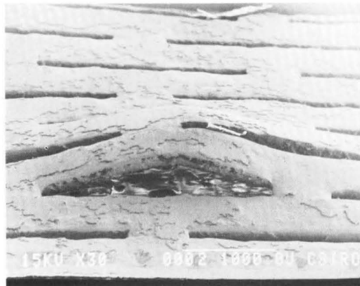
Fig. 8. Chrome-nickel screen showing slot distortion over the backing screen (Magnification \times 30 )
