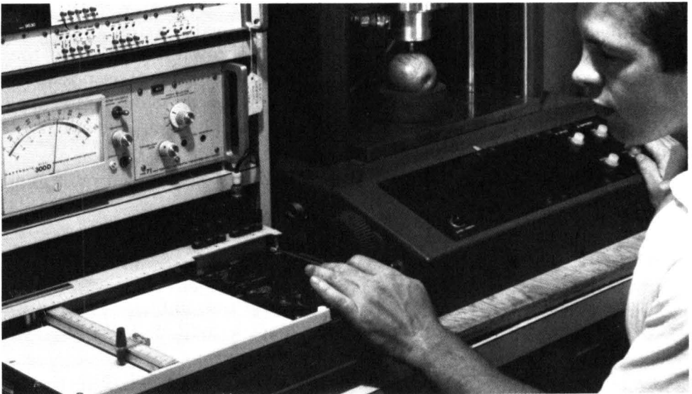
FIG. 1. QUASI-STATIC FIRMNESS MEASUREMENT USING A 1.11 CM (7/16 IN.) MAGNESS TAYLOR PROBE
