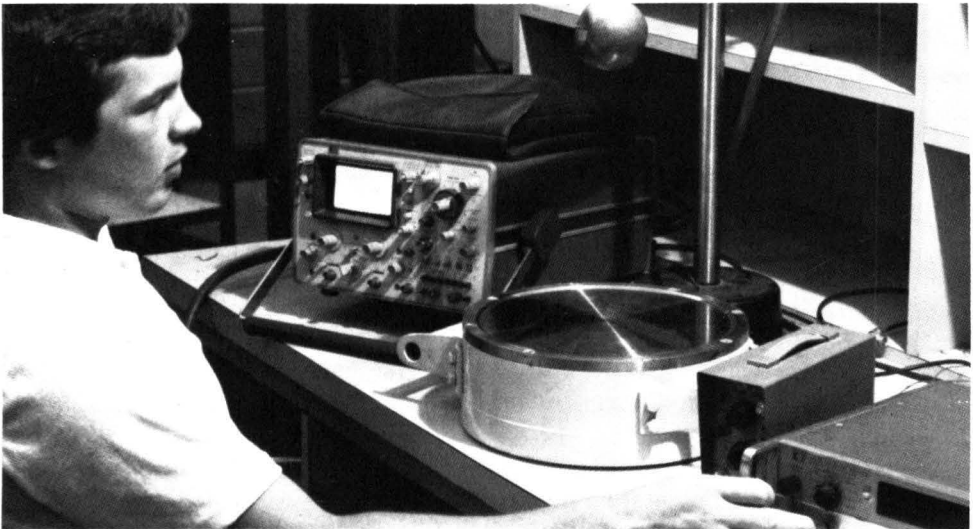
FIG. 2. IMPACT TESTING USING A 25.4 cm CROP ON A FLAT STEEL PLATE
