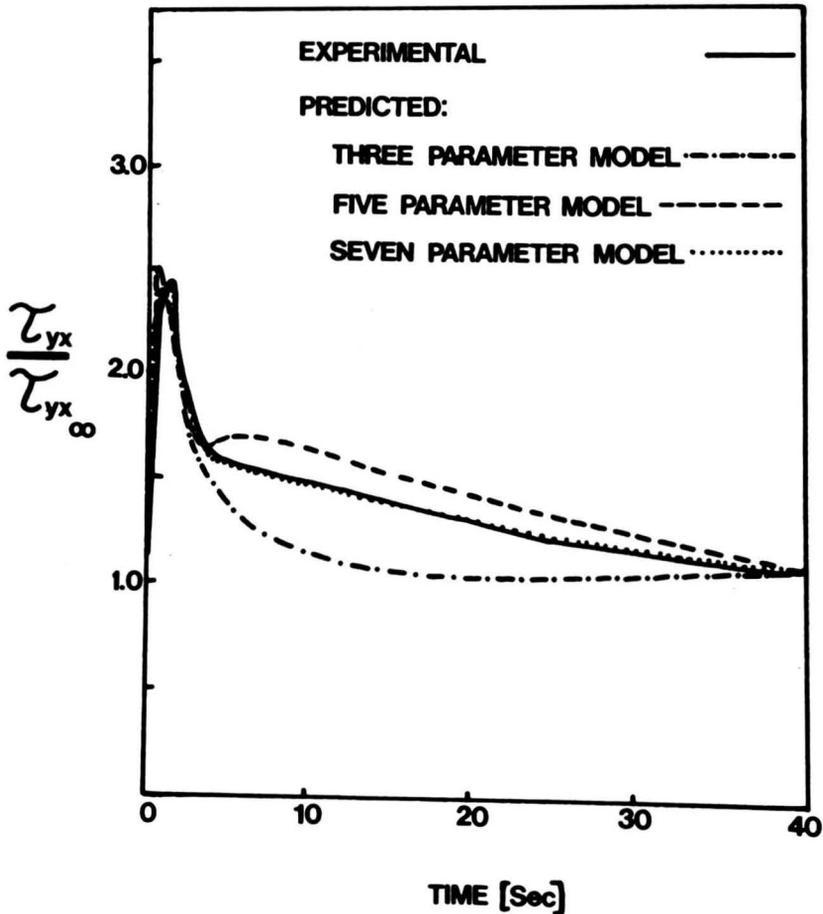
FIG. 5. SHEAR STRESS DEVELOPMENT OF PEANUT BUTTER AT  $\dot{\gamma} = 10 \text{ S}^{-1}$
