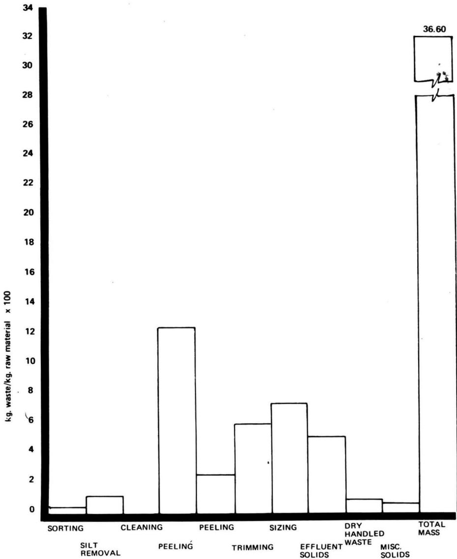
FIG. 2. MAGNITUDES OF PRODUCT LOSS FOR UNIT OPERATIONS FOR POTATO PROCESSING
