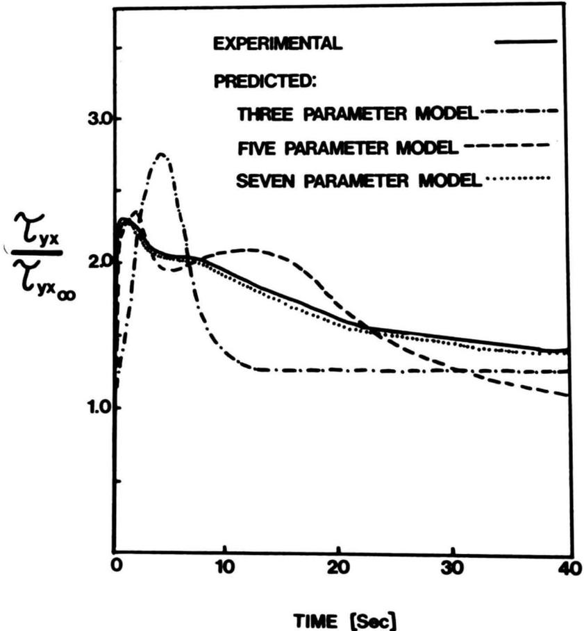
FIG. 1. SHEAR STRESS DEVELOPMENT OF STICK BUTTER AT  $\dot{\gamma} = 10 \text{ S}^{-1}$
