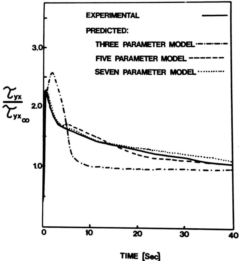
FIG. 4. SHEAR STRESS DEVELOPMENT OF TUB MARGARINE AT  $\dot{\gamma} = 100 \text{ S}^{-1}$
