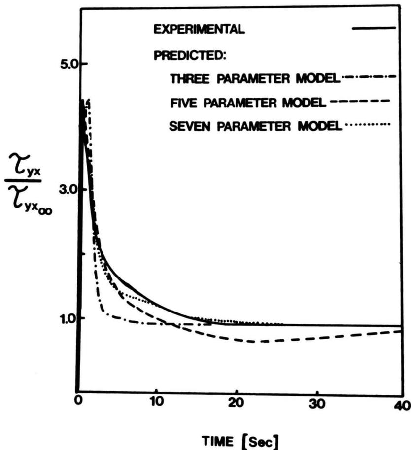
FIG. 6. SHEAR STRESS DEVELOPMENT OF PEANUT BUTTER AT  $\dot{\gamma} = 100 \text{ S}^{-1}$
