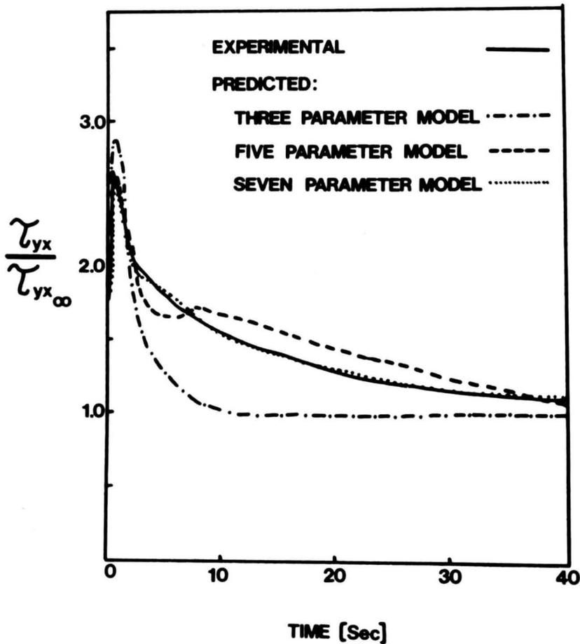
FIG. 2. SHEAR STRESS DEVELOPMENT OF STICK BUTTER AT  $\dot{\gamma} = 100 \text{ S}^{-1}$
