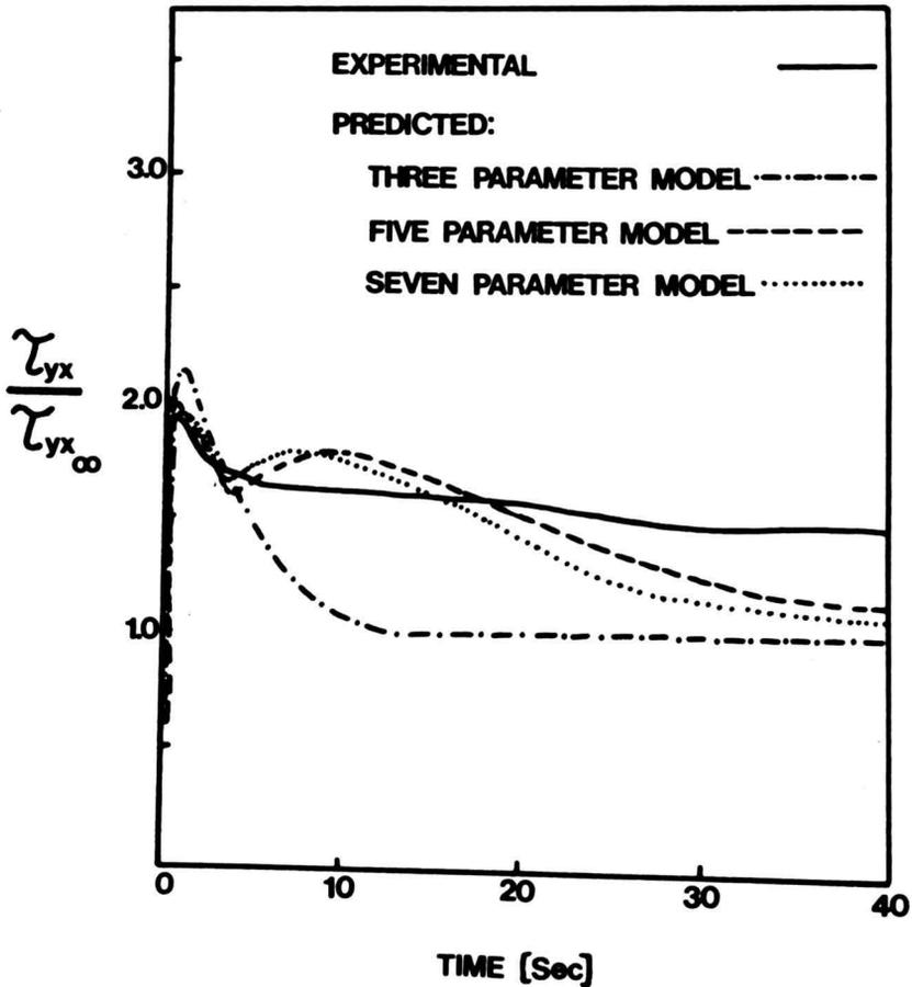
FIG. 7. SHEAR STRESS DEVELOPMENT OF CANNED FROSTING AT  $\dot{\gamma} = 10 \text{ S}^{-1}$
