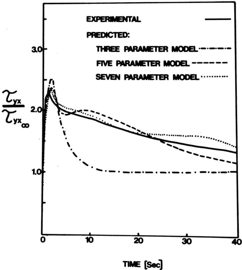
FIG. 3. SHEAR STRESS DEVELOPMENT OF TUB MARGARINE AT  $\dot{\gamma} = 10 \text{ S}^{-1}$
