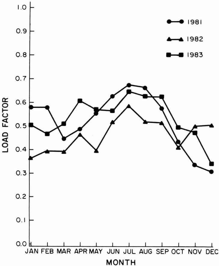
FIG. 3. ELECTRICAL LOAD FACTORS OF THE FISH PLANT FROM 1981 TO 1983
