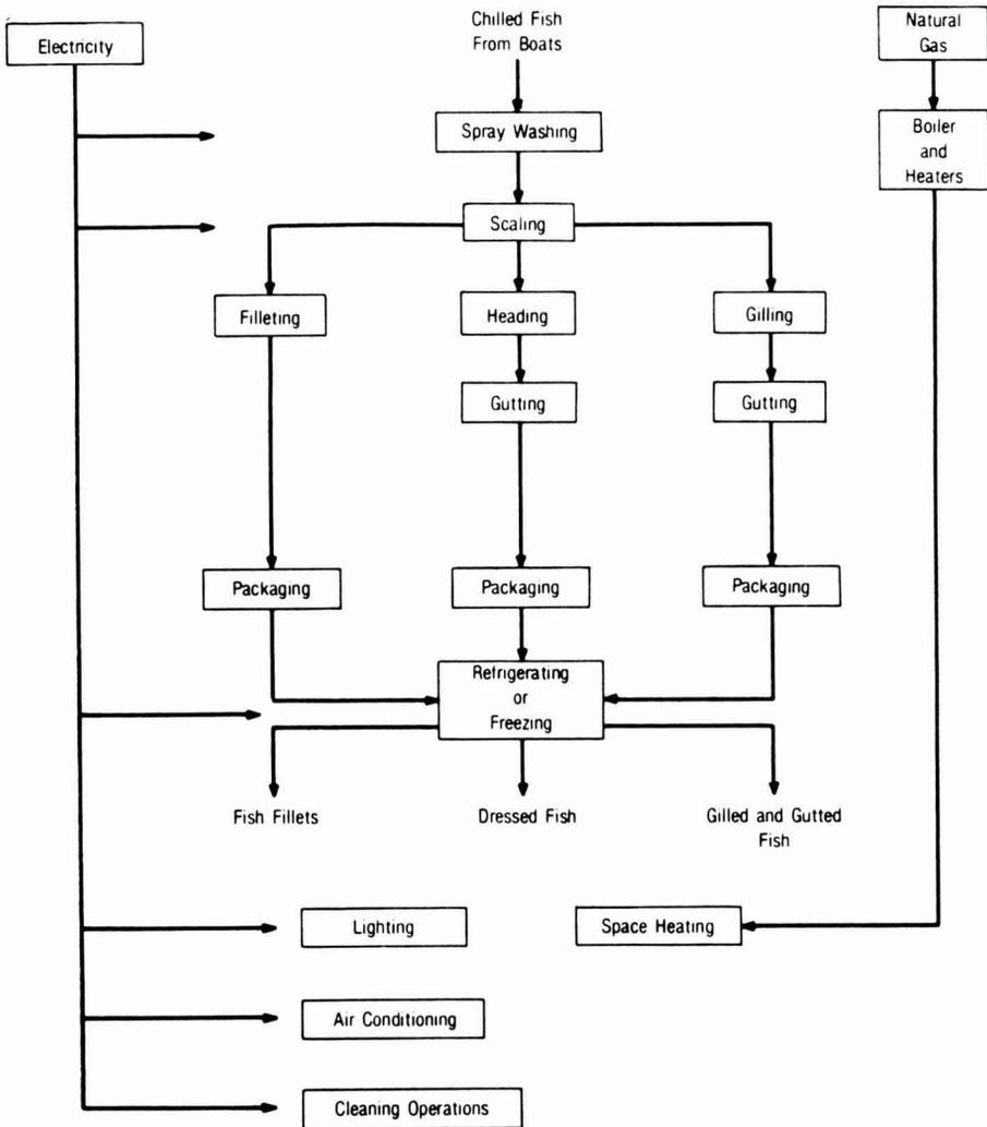
FIG. 1. PROCESS FLOWCHART FOR THE PRODUCTION OF FRESH AND FROZEN FISH PRODUCTS AND RELATED ENERGY INPUTS.
