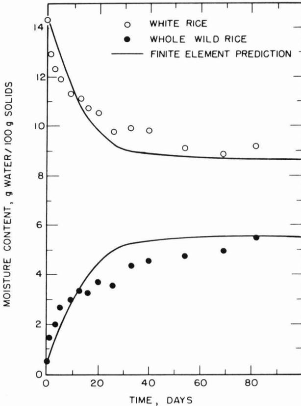
FIG. 3. ACTUAL MEASURED MOISTURE CONTENTS VERSUS TIME FOR THE COMPONENTS OF A WHITE RICE-WHOLE RICE MIXTURE COMPARED TO THE FINITE ELEMENT PREDICTION
