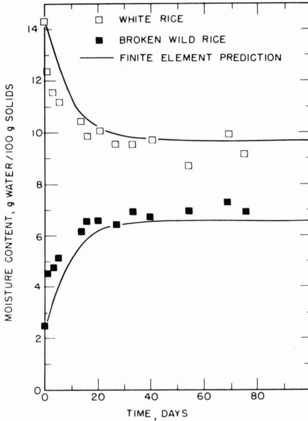
FIG. 5. ACTUAL MEASURED MOISTURE CONTENT VERSUS TIME FOR THE COMPONENTS OF A WHITE RICE-BROKEN WILD RICE MIXTURE COMPARED TO THE FINITE ELEMENT MODEL
