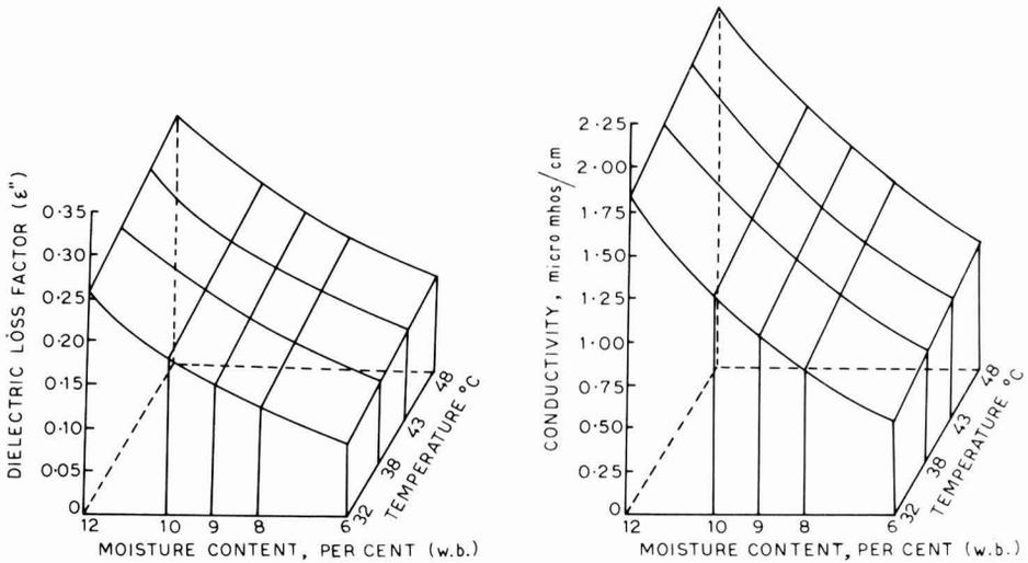
FIG. 4. RESPONSE SURFACES FOR DIELECTRIC LOSS FACTOR AND A.C. CONDUCTIVITY AT A BULK DENSITY OF 360 kg/m<sup>3</sup>
