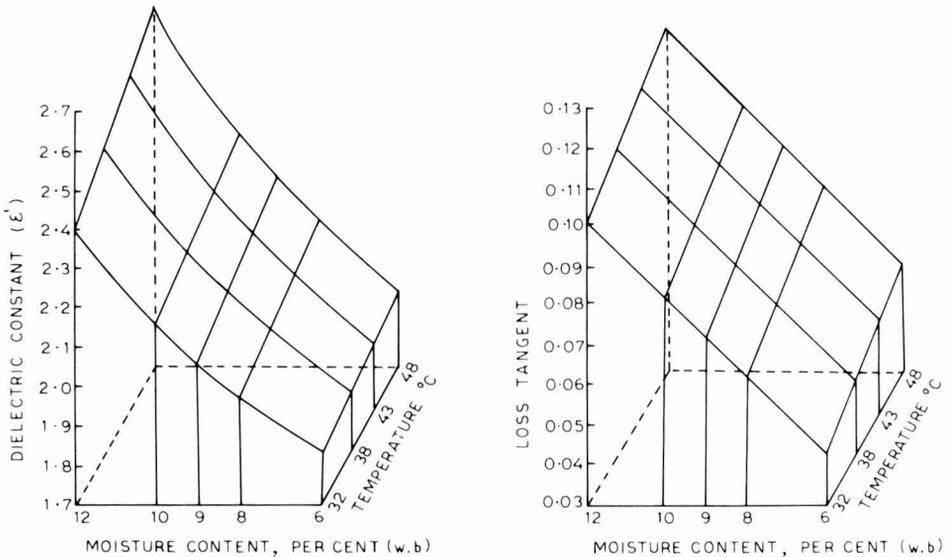
FIG. 3. RESPONSE SURFACES FOR DIELECTRIC CONSTANT AND LOSS TANGENT AT A BULK DENSITY OF 360 kg/m<sup>3</sup>
