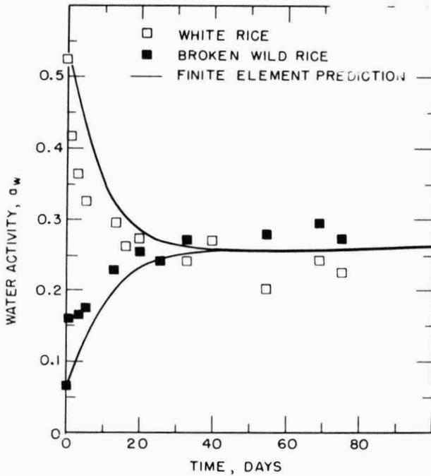
FIG. 6. CHANGE IN WATER ACTIVITY (as evaluated from the GAB isotherm) FOR A WHITE RICE-BROKEN WILD RICE MIXTURE (from Fig. 5) AS A FUNCTION OF TIME COMPARED TO THE FINITE ELEMENT PREDICTION
