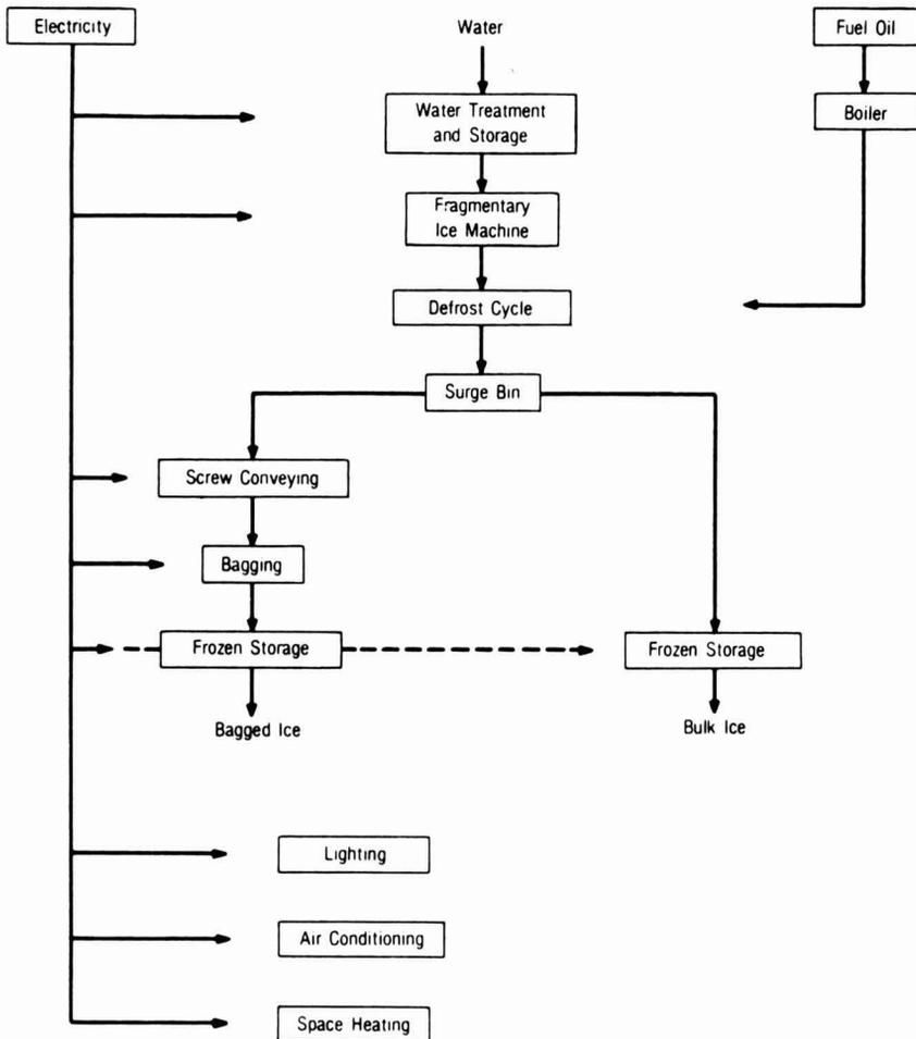
FIG. 2. PROCESS FLOWCHART FOR THE MANUFACTURE OF BULK AND BAGGED ICE AND RELATED ENERGY INPUTS
