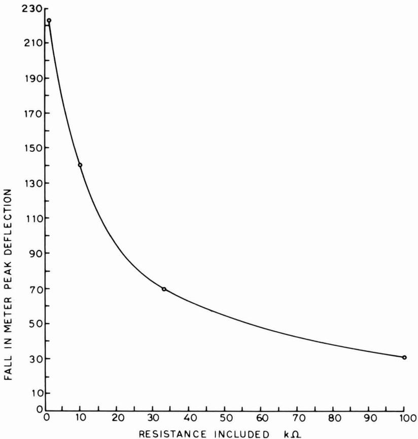
FIG. 2. CALIBRATION CURVE AT 13.56 MHz FOR EVALUATING THE EQUIVALENT PARALLEL RESISTANCE OF THE SAMPLE
