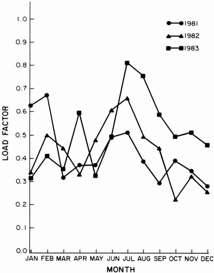
FIG. 5. ELECTRICAL LOAD FACTORS OF THE ICE MANUFACTURING PLANT FROM 1981 TO 1983
