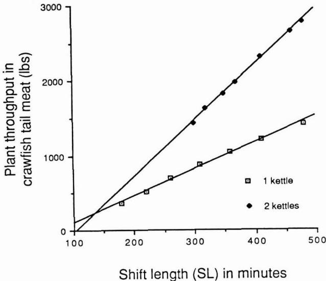
FIG. 4. PLANT THROUGHPUTS CORRESPONDING TO DIFFERENT SHIFT LENGTHS AND NUMBER OF KETTLES
