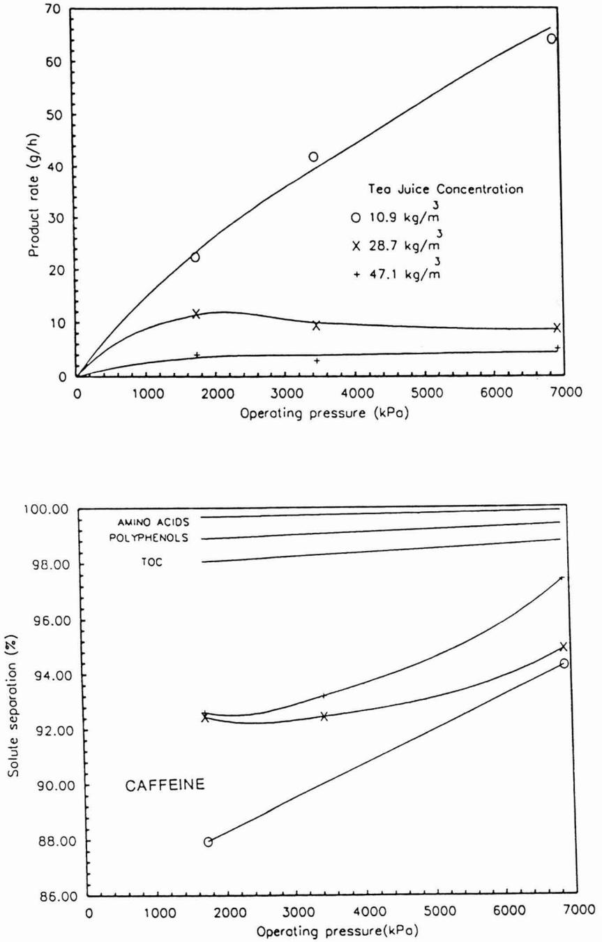
FIG. 4. SEPARATIONS OF VARIOUS TEA JUICE COMPONENTS AND PRODUCT RATE FOR DIFFERENT FEED TDS VALUES AND OPERATING PRESSURES
