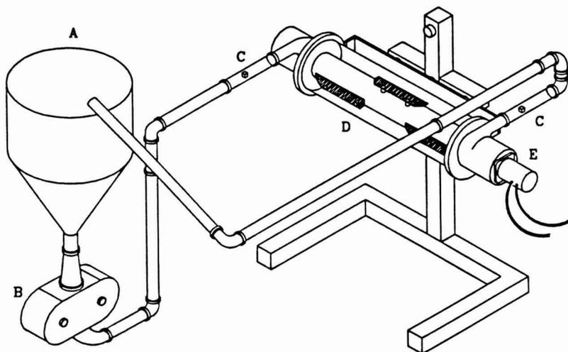
FIG. 1. SCHEMATIC DIAGRAM OF A MODEL HORIZONTAL SSHE
