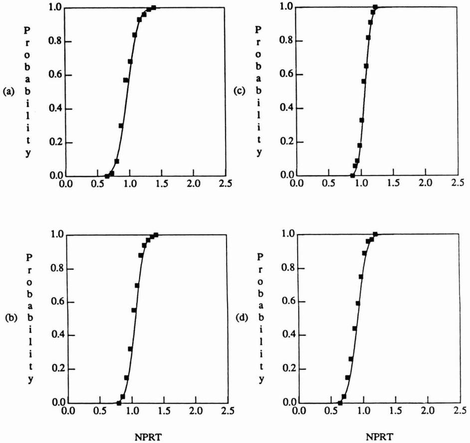
FIG. 2. NORMAL CUMULATIVE DISTRIBUTION FUNCTION OF NORMALIZED PARTICLE RESIDENCE TIME IN A HORIZONTAL SSHE
