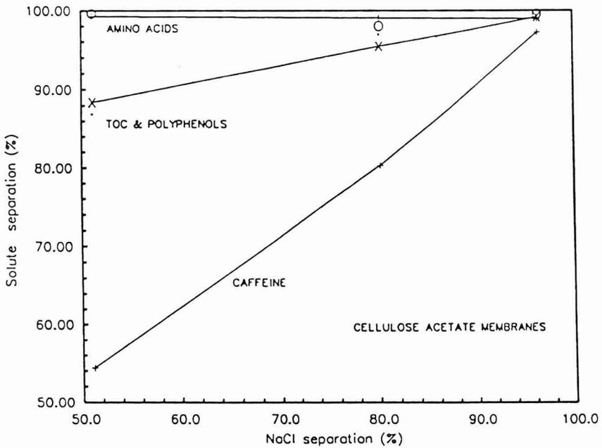
FIG. 2. SEPARATIONS OF VARIOUS TEA JUICE COMPONENTS AND PRODUCT RATE VERSUS SODIUM CHLORIDE SEPARATION
