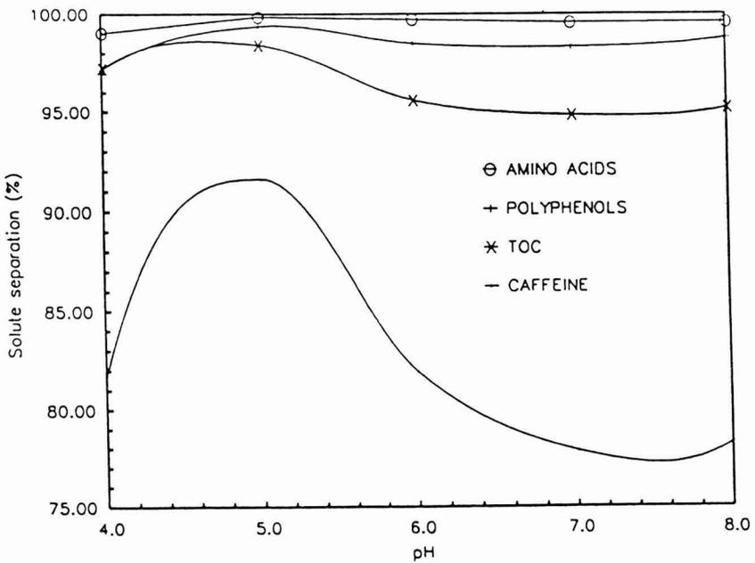
FIG. 3. SEPARATIONS OF VARIOUS TEA JUICE COMPONENTS AND PRODUCT RATE FOR DIFFERENT FEED pH
