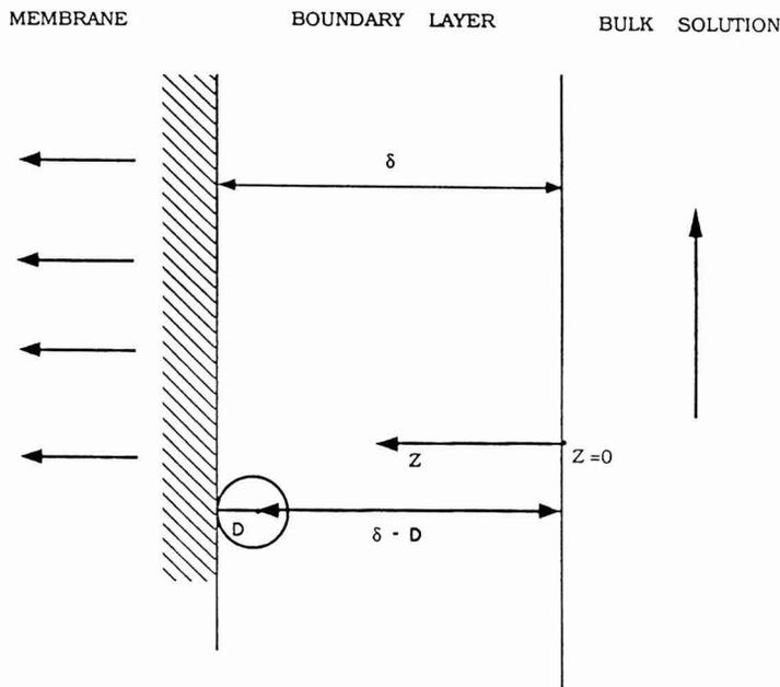
FIG. 1. SCHEMATIC DIAGRAM OF BOUNDARY LAYER
