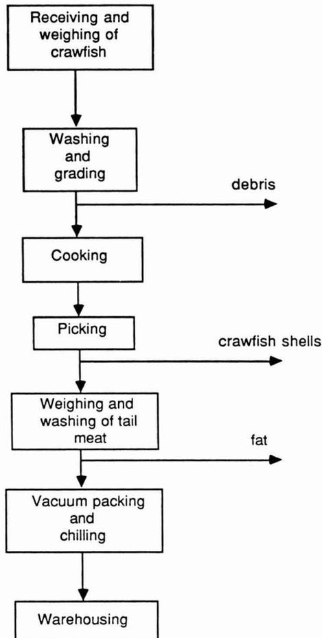
FIG. 1. FLOWCHART OF CRAWFISH PROCESSING OPERATIONS
