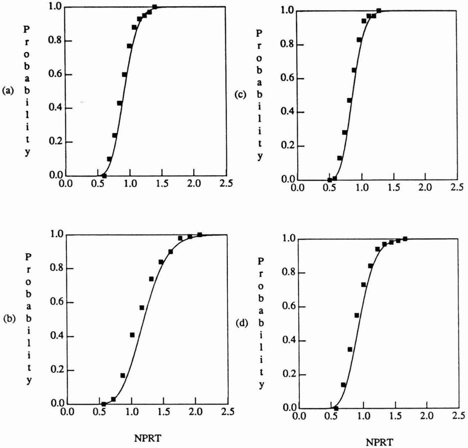
FIG. 3. GAMMA CUMULATIVE DISTRIBUTION FUNCTION OF NORMALIZED PARTICLE RESIDENCE TIME IN A HORIZONTAL SSHE
