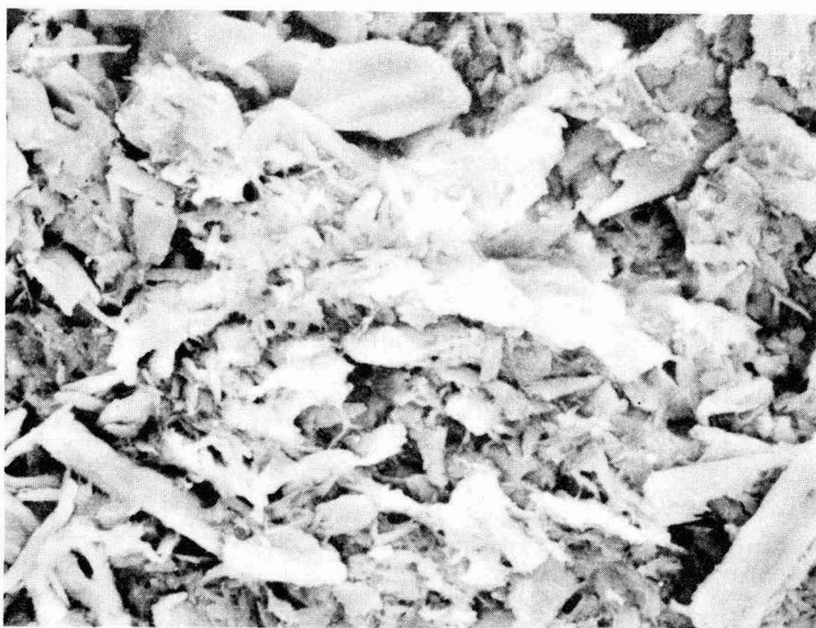
FIG. 1. SCANNING ELECTRON MICROSCOPE VIEW OF 4.5% LINOLEIC ACID, 15% AVICEL FREEZE DRIED EMULSION (COATED WITH GOLD) (400X)
