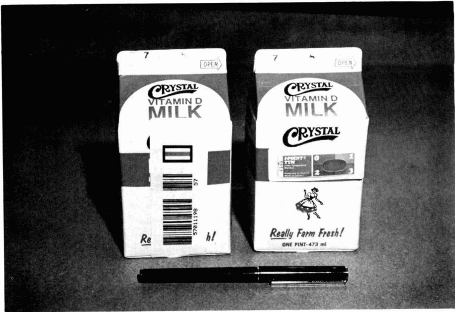
FIG. 1. LIFELINE FRESHNESS MONITOR MODEL 57 (LEFT) AND I-POINT TIME/TEMPERATURE MONITOR MODEL 2140 (RIGHT) PLACED ON 1-PINT CARTONS OF PASTEURIZED MILK
