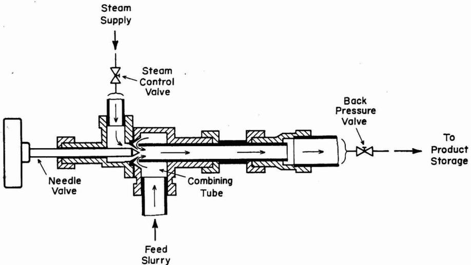
FIG. 2. DESIGN OF THE HYDROHEATING VALVE
