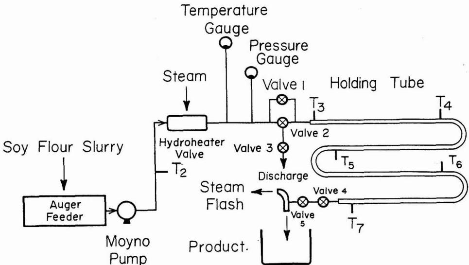
FIG. 1. RAPID HYDRATION HYDROTHERMAL JET COOKER AND FLASH COOLER (Johnson 1978).
