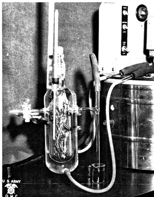
FIG. 1. Sample cell for gas chromatographic analysis.
