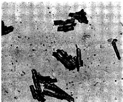
Fig. 1. Sodium glucose sulfonate crystals ( \times 44 ).
