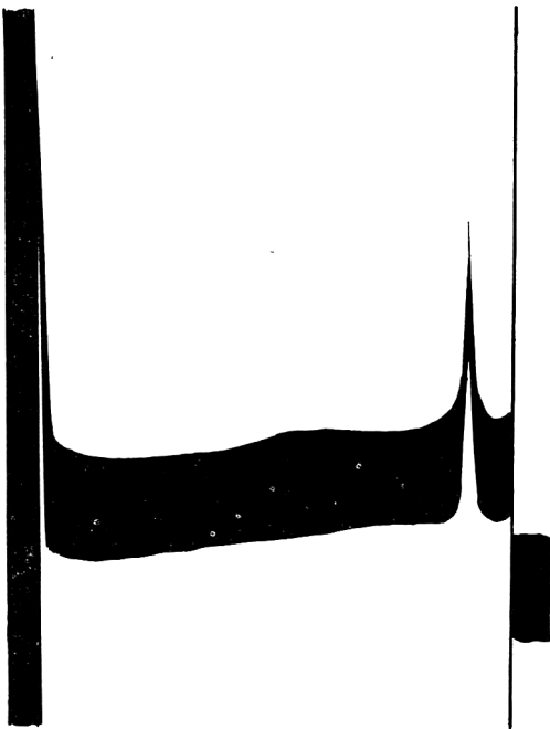
FIG. 6. Ultracentrifugal run of myosin A prepared from fresh beef muscle. Protein conc. 2.0 mg/ml, pH = 6.60, 0.5M NaCl, 16 min.
