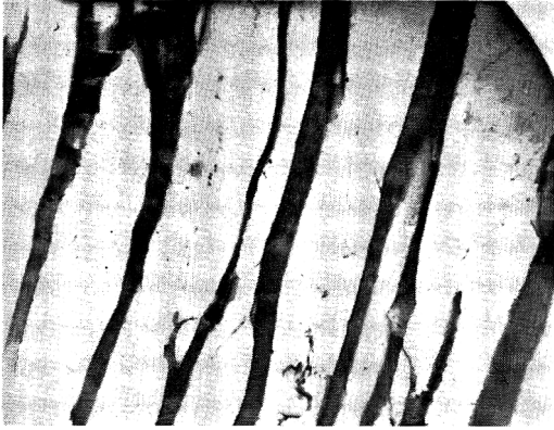
Fig. 1. Longitudinal section of fish frozen at the critical speed, about 60 min. Light areas represent ice. Each cell contains just one column of ice growing up the center. On left is the end of one ice crystal: it is here that salts are believed to accumulate and cause accelerated denaturation. Distance left to right represents about 1 mm of original tissue.
