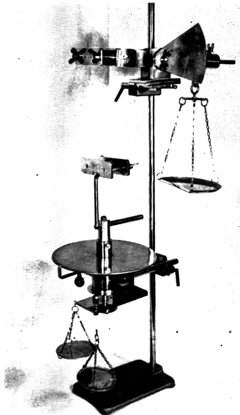
Fig. 3. Original laboratory tool to measure the changes of the torsion elasticity of muscle.
