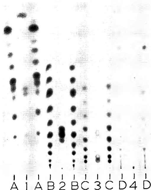
Fig. 1. Thin-layer chromatoplate of carbonyl compounds as their 2,4-dinitrophenylhydrazones comparing reference derivatives with those from liquor (Accra). A) alk-2-enals C_3 through C_{13} ; B) alkanals C_1 through C_{10} ; C) alk-2-enals C_3 through C_{10} ; D) alk-2,4-dienals C_3 through C_{16} (less C_8 , C_{13} and C_{15} ). 1, 2, 3, and 4 are respectively the fractions from liquor corresponding to the reference mixtures A, B, C, and D.
