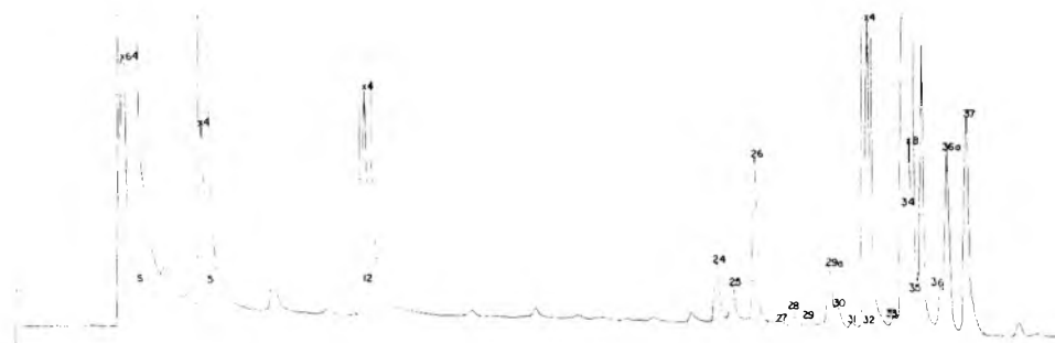
Fig. 4. Chromatogram of essence obtained by extraction of commercial deaerator effluent.
